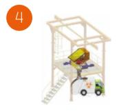
Waste Discharging Sterilized waste is discharged automatically to truck or container.
