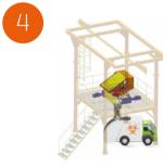
Waste Discharging Sterilized and shredded waste is discharged automatically to truck or container.
